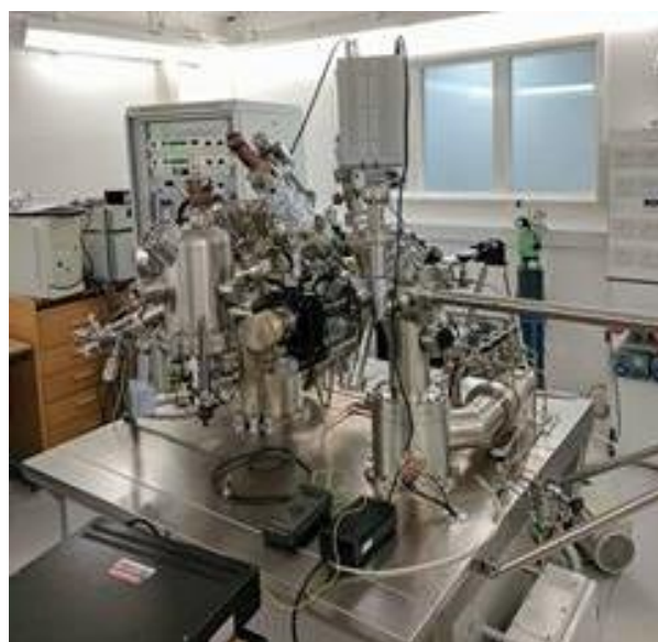
UHV chamber equipped with an Omicron variable-temperature STM, LEED, and a thin-film growth facility.
